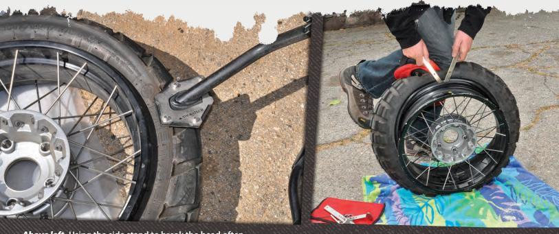
**Above left** Using the side stand to break the bead often does the job. It certainly has the leverage. But if you don't have a center stand to balance the bike on, the maneuver can be difficult, if not impossible, to pull off.
