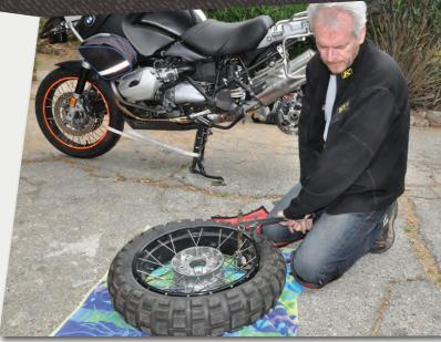
Using a tool like *BestRest Product's BeadBrakR* makes one of the most difficult in the field tasks of breaking tire beads not just easier, but possible.
